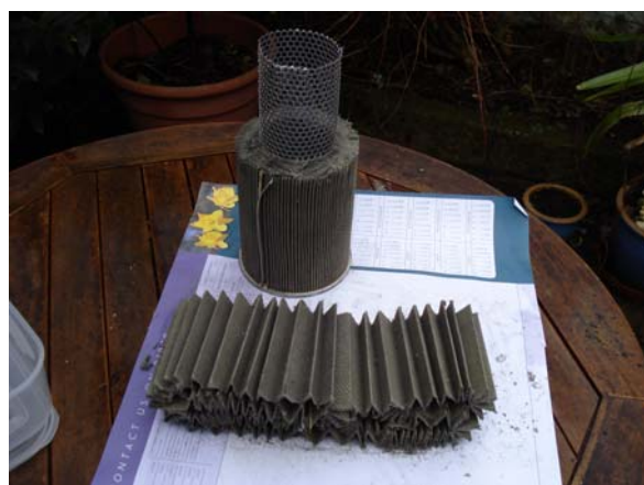
Fig 1. Ambulance air filter from Gaza before and after cutting up.
